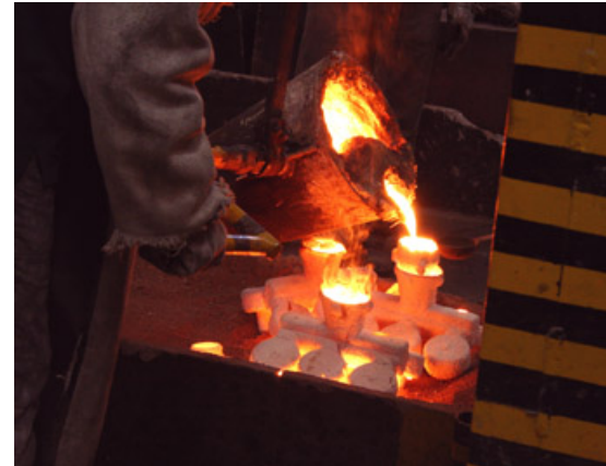
Pouring the alloy into the mold
